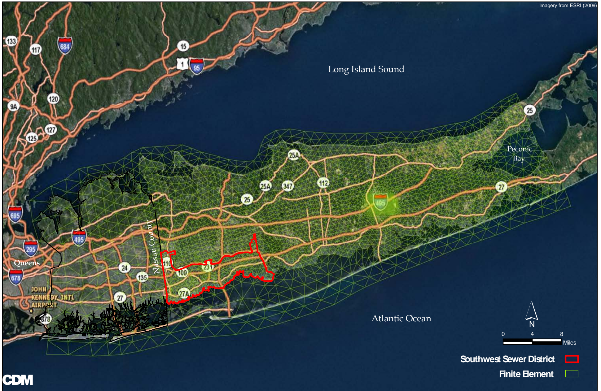
Suffolk County Department of Public Works Bergen Point WWTP Outfall Replacement Project Finite Element Grid for Suffolk County Regional Groundwater Model
