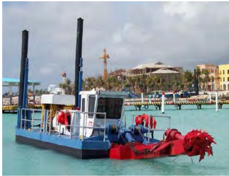
Figure 3-18 Conventional Hydraulic Dredge ( Courtesy of Ellicott Dredge )
