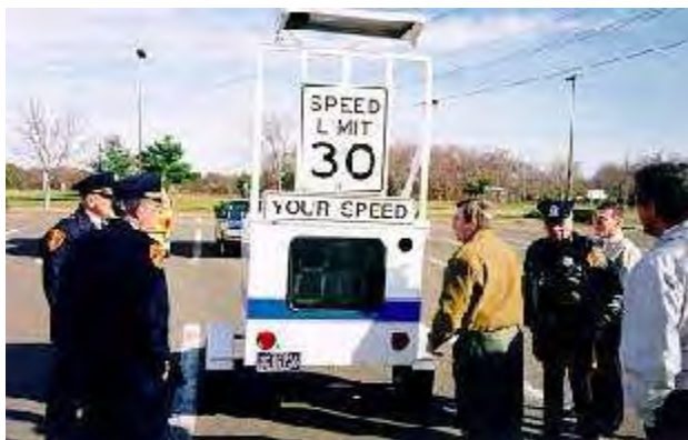
Figure 18 A Smart Machine which is a radar unit that shows your speed.
