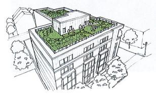
**GREEN ROOF** – A building roof that is engineered to be covered with low-maintenance growing plants that insulate in winter, cool the building in summer, reduce solar absorption, reduce precipitation run-off surfaces, and improve interior Heating, Ventilating and Air Conditioning (HVAC) efficiency.
