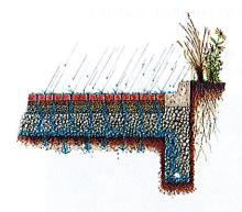
POROUS/PERMEABLE PAVEMENT — A hard surface with load bearing capacity engineered to allow for the passage of water through pores. Porous pavements are often underlain by carefully engineered layers of crushed rock, fabric filter cloth, piping, or drains. Types of porous pavement may include paving blocks with open corners, lattices, or edges or asphalt/concrete mixes without fine sediments.
