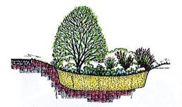
**BIO-RETENTION BASIN** — An area designed to accept and retain stormwater, to slow or block either its discharge to surface water or its recharge to groundwater, to lessen erosion, allow for filtering of sediments, plant root uptake of nutrients, and biologically control the water. It may be equipped with various overflows or high water level bypasses to transport amounts of water exceeding its holding capacity.
